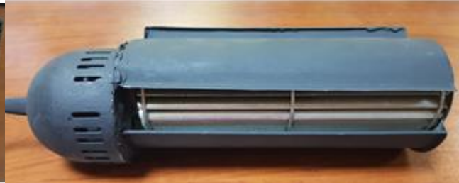
Figure 5. Wind exit unit of wind turbine
